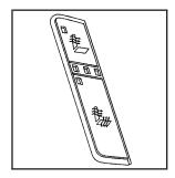
Your vehicle may have heated front seats. The controls are located on the driver's and passenger's doors, near the door handle.
